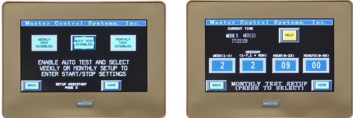
To enable, press the AUTO TEST button. Then select either the monthly or weekly test, and enter the time you would like the test to automatically occur.
